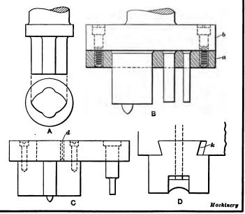
Fig. 19. Different Types of Punches
